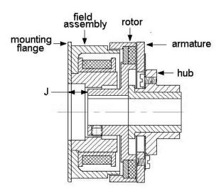
FL series power-on clutches are used to couple two parallel shafts. The armature hub assembly is mounted to the same shaft as the rotor assembly. The armature hub accommodates a pulley, gear, sprocket, etc., to transmit torque. The field assembly is mounted to a bulkhead that is perpendicular to the clutch shaft. Typical FL clutch installations require a coupling between the drive shaft (motor shaft) and the driven shaft (clutch shaft) to accommodate assembly.
